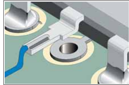
Figure 12 Acceptable Wire soldered to lifted component lead. +
